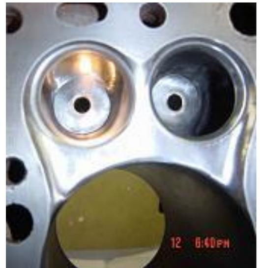
**PS: Glob-o-Matic:** Barney Navarro and I talked about custom guides and intake port flow -- he mentioned that he has seen guys weld a big glob of brass or even lead to the tops of the guides, then hand blend the port "turn" into this material. The goal was to help the air flow make the turn and not slam into the valve pocket wall! Cool Stuff . . . just wish I had more time to play and try this!
