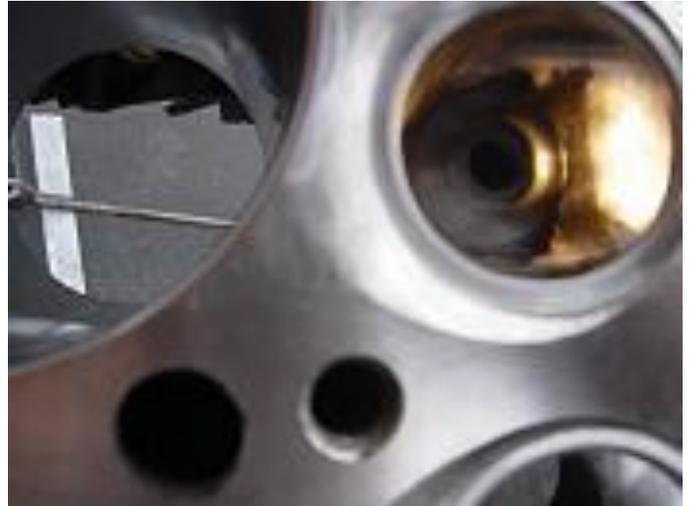
**Custom Fitting Guides to Individual Ports:** This example is on the 59L competition engine - where I wanted to blend the guide into the port shape as close as possible to the port floor. Every guide is individually fitted - and then it is indexed/pinned to keep the orientation. These are prototypes, will probably replace the bronze liner to stick up the full-length when I'm done.
