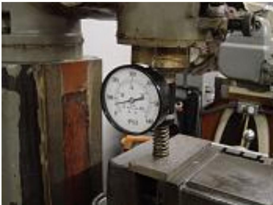
**3) Sample Spring Pressures and Flathead Myths:** Here are some numbers to review on spring type, pressure and installed heights. I wanted to check it with a reasonable seat pressure and a "nose" pressure - assuming a Potvin 3/8 cam - .375 or so lift (gross).
