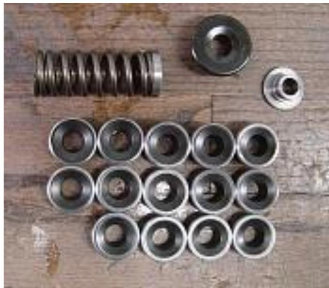
Here is the complete assembly - ready to go . . . nice and clean. I still needed one thick shim .060 and one .015 shim . . . better than 5!
